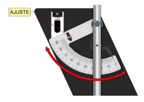
Turn the angle marker pointer until it touches the ballistic pendulum arm. If angle is not  $0^{\circ}$ , loosen the screw and adjust the scale to  $0^{\circ}$ .
