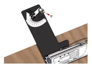
Remove the PENDULUM'S THUMB SCREW.
