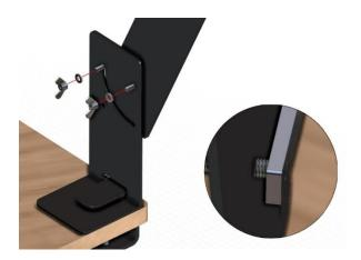
Fasten the washers and butterfly nuts. Do not tighten until the end, it is necessary to leave a gap to fit the cannon.
