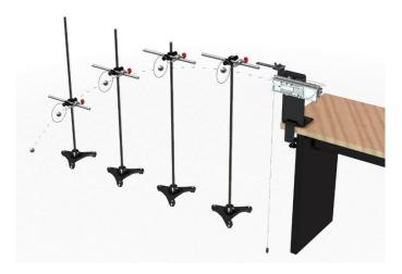
**15.** Prepare the projectile launch with the plastic ball in the first stage. Fire the launch and verify if the projectile has passed through the rings without touching them.
