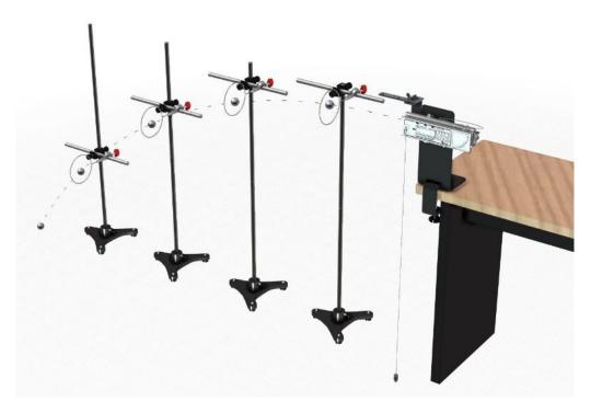
**14.** Prepare the projectile launch with the plastic ball in the first stage. Fire the launch and verify if the projectile has passed through the rings without touching them.
