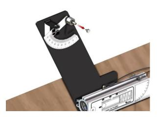
Remove the PENDULUM'S THUMB SCREW.
