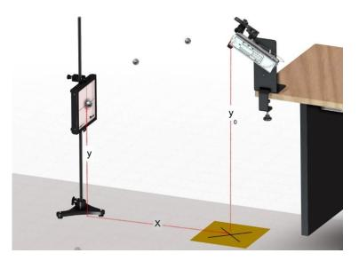
**3.** Using the plumb bob, affix a paper sheet on the floor aligning with the cannon mouth.
