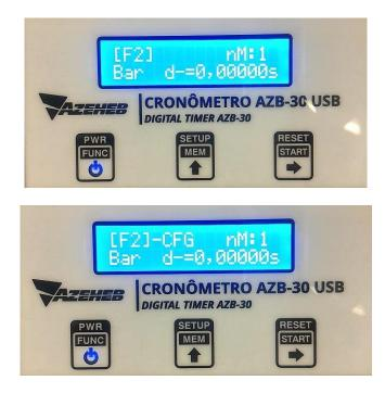
To select the desired measurement type, press the SETUP key for 2s to enter the configuration mode. In the configuration mode, use the START / RESET key to navigate among the configuration parameters. To change a selected parameter use the SETUP / MEM  $\uparrow$  keys. After setting the function, press the FUNC key to save the selected parameters.
