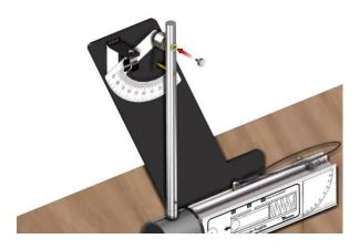
Reattach the PENDULUM'S THUMB SCREW.
